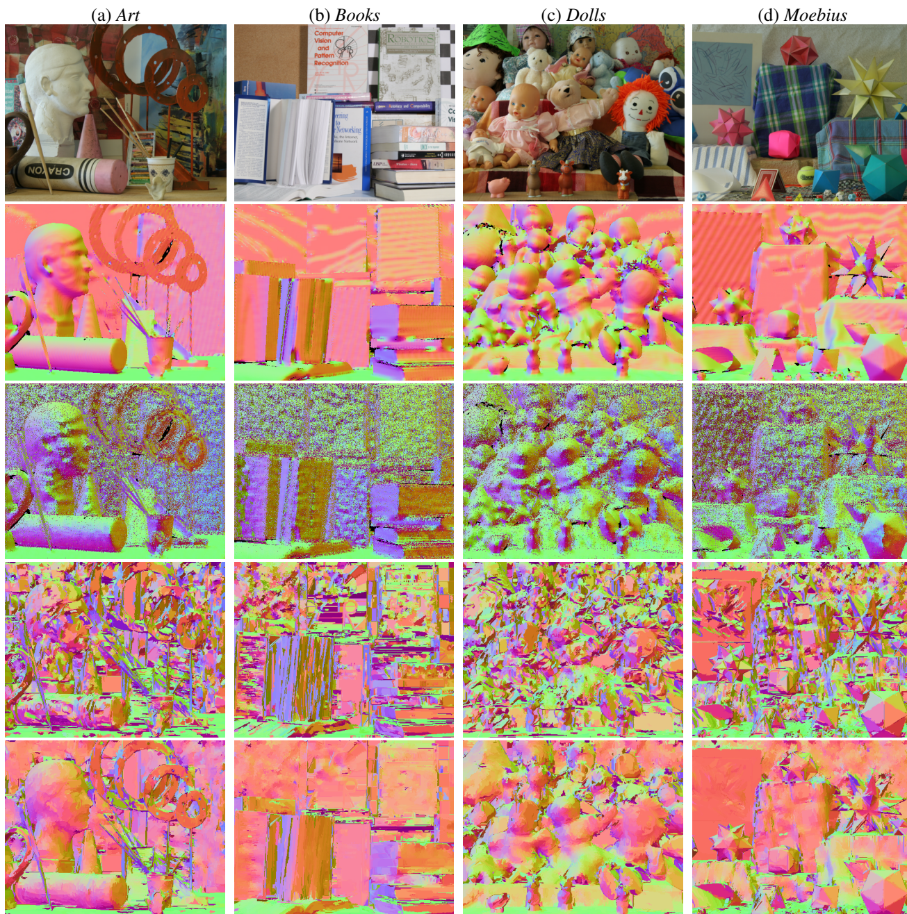
Figure 3. Orientation correction results represented as normal maps. Color images of the scenes, normal maps of smooth high-resolution depth images, normal maps of noisy high-resolution depth images, normal maps calculated by PCA and our color heuristic PCA on each superpixel, and the corrected normal maps by our proposed method. (noise coefficient k = 3.0 \times 10^{-6} , magnification factor \times 4 \times 4 )
