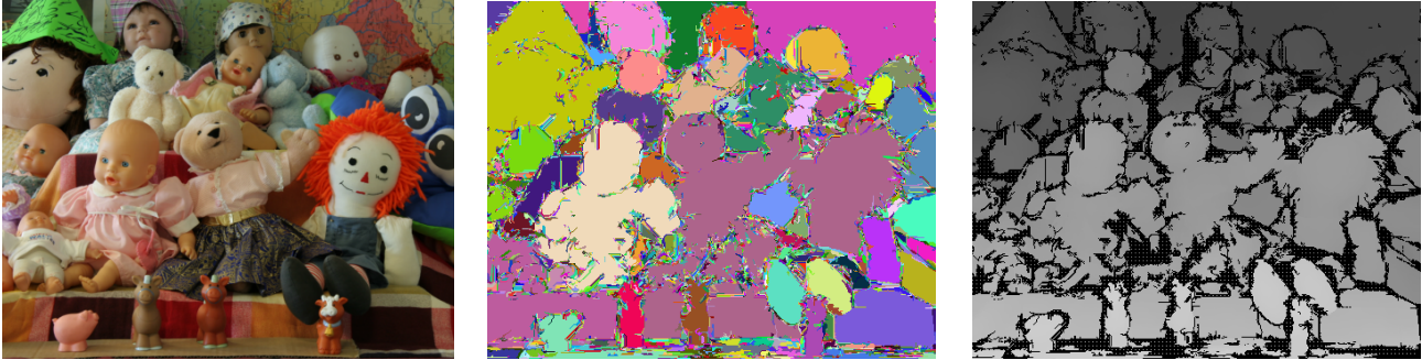
Figure 2. Left: Color image. Middle: Resulting smooth surface segmentation. Right: Interpolation result. (magnification factor x16).
